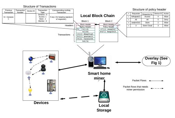
Fig. 2. Overview of the Smart home: The smart home consists of IoT devices, local storage (see section II.D), the miner (see section II.C), and the local BC (see section II.B).
