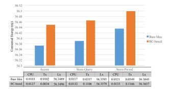
Fig. 4. Evaluation of energy consumption in different traffic flows.
